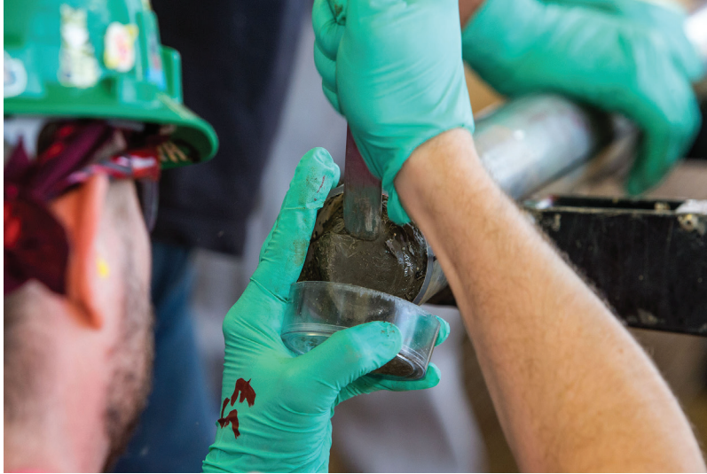
Trimming the end of an Expedition 355 core section on the catwalk.
